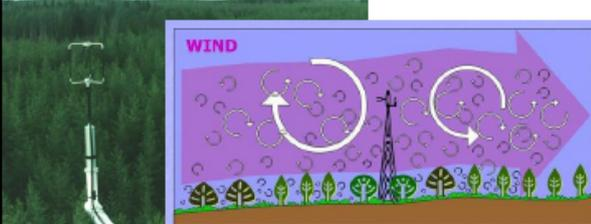
The diagram shows a forest with a measurement tower. A large purple arrow labeled 'WIND' indicates the direction of air flow. White circular arrows show the vertical mixing of air, representing the eddy covariance process. The ground is brown, and the forest is green.
